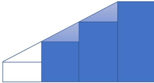
Figure 6.1 Idea of transition part between aluminium honeycomb and 3D printed structure
