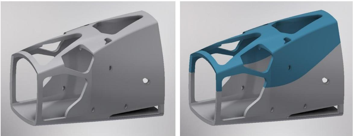
Figure 5.9 New model base on the left and divided model on the right
