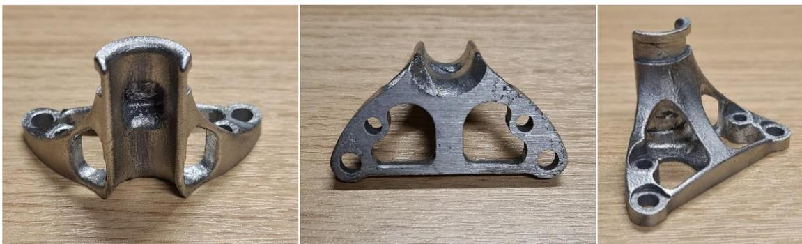
Figure 4.8 Guidance block near engine for wire bypass. Author's photos
