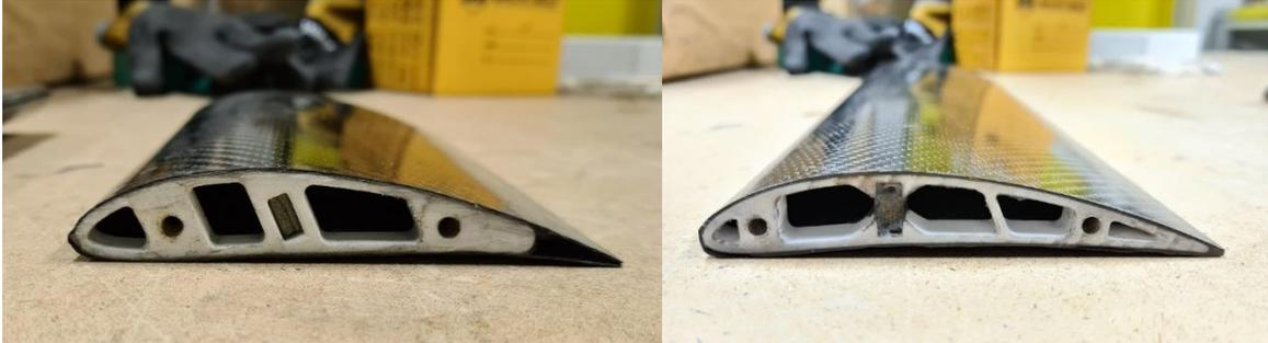
Figure 4.9 3D printed structures inside formula car wings. Author's photos
