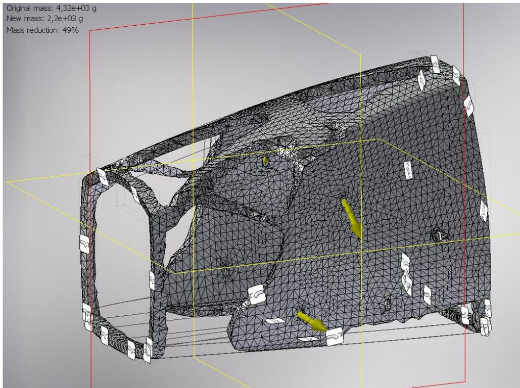
Figure 5.6 Topology optimization results, isometric view
