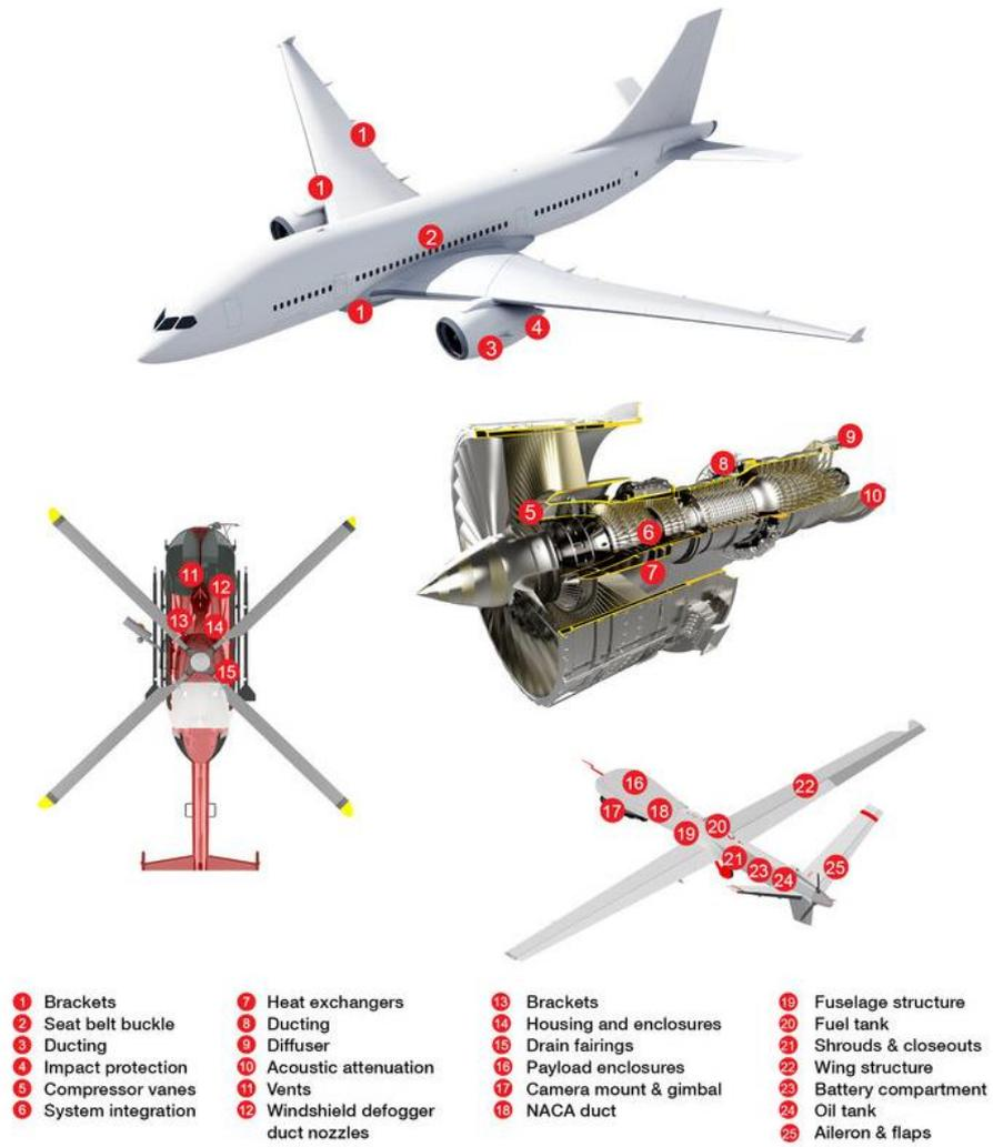
Figure 3.14 Aerospace AM applications [30]
