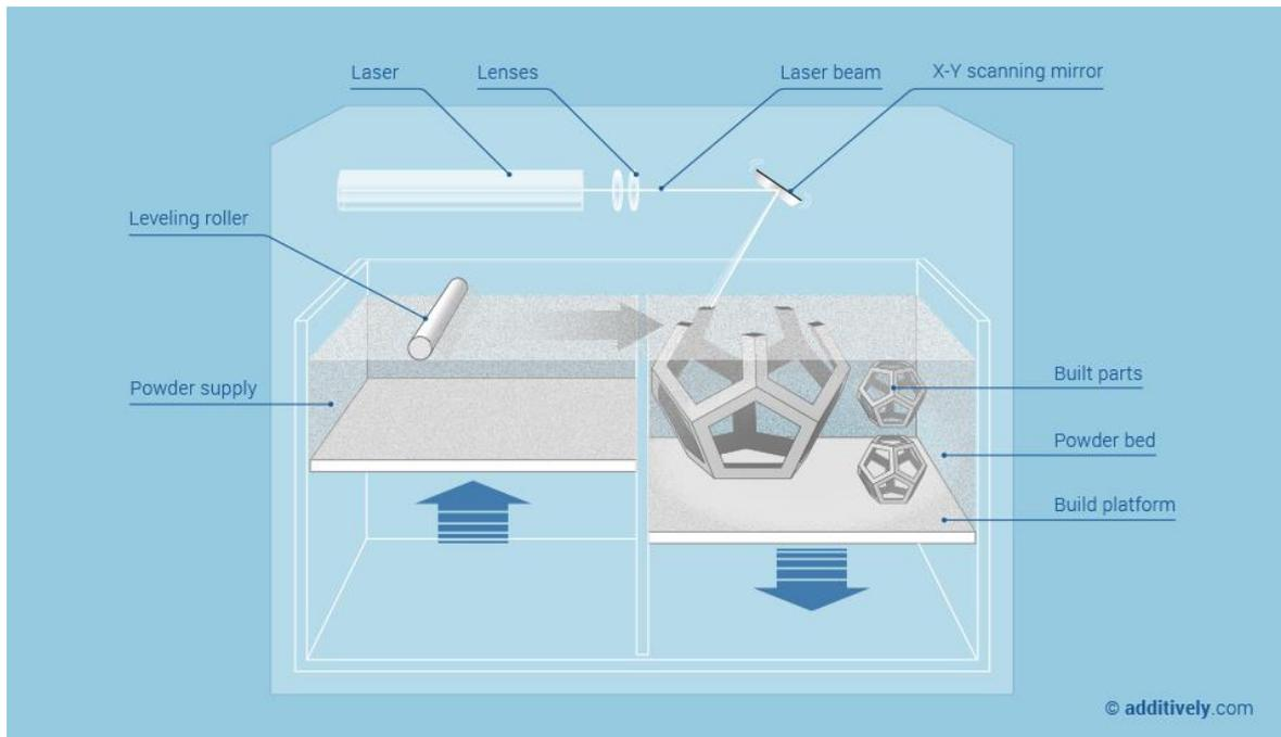
Figure 3.4 SLS printer [16]
