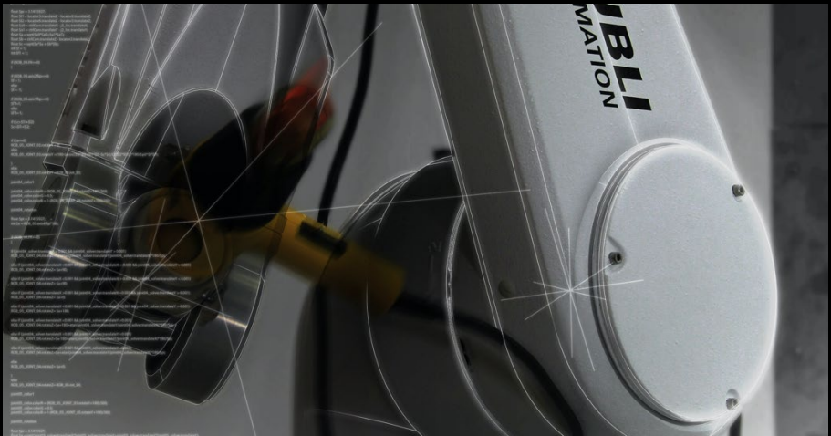
Fig. 21. A regular heat gun used as an end of arm tool for the sPhysical project. Team: Erin Besler, Eugen Kosgoron, Siim Tuksam and Peter Vikar. 2011 winter term in Studio Testa, Sci-Arc, Los Angeles.
